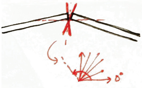
Figure 3.3.1: for 100 plates; 100 different angles. Therefore, find that 1 connection with changeable angles.
