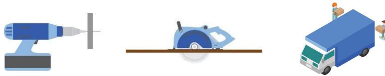
Figure 15: Pre-construction processes: cut planks and mark/drill intersections (left), cut wood in-ground foundation anchors (center), transport to site in a single trip in a small van (right).
