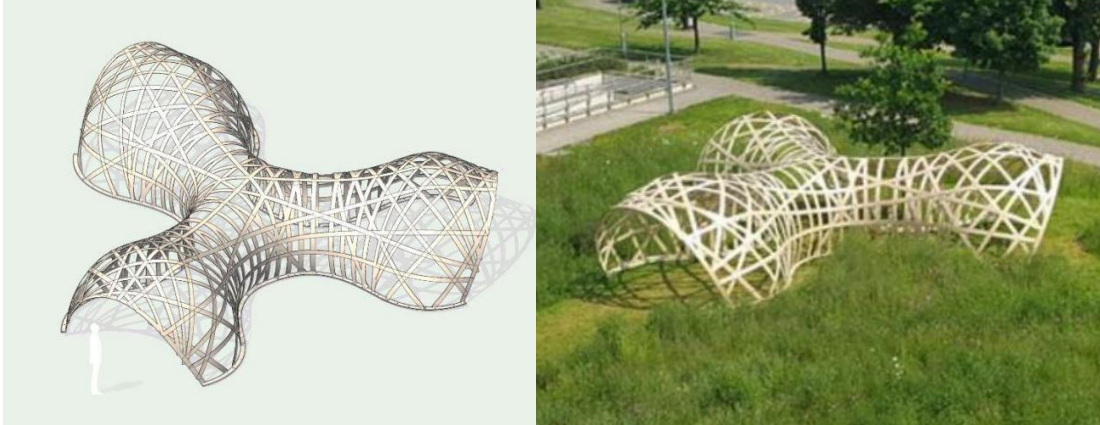
Figure 5: Final digital geometry (left) and the erected structure (right) [11]
