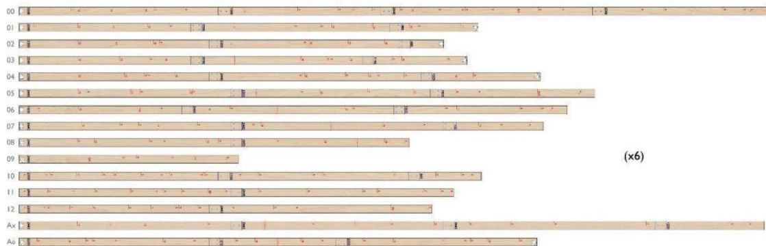
Figure 6: The unique set of 15 linear plywood planks, a total of 6 sets were required [11].
