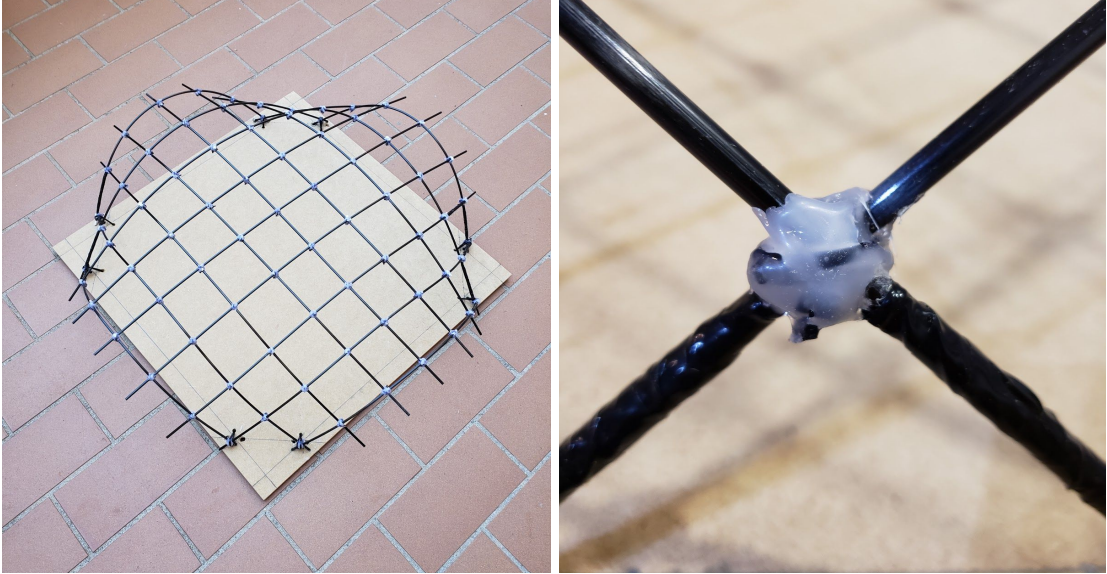
Figure 34 : Small Gridshell assembled and detail of the joint
