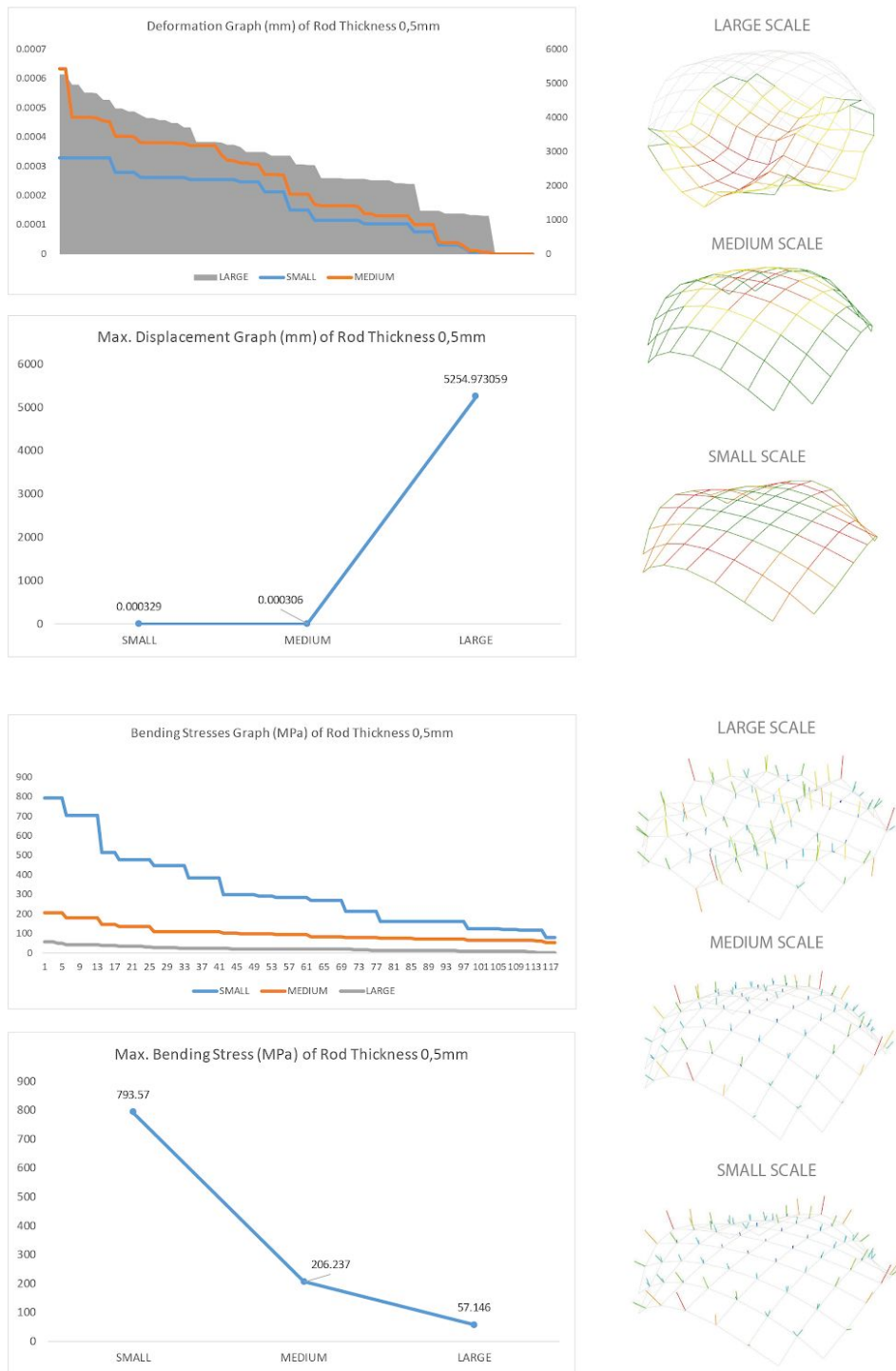
Figure 25 : Displacement and Bending Stresses Analysis with 0,5mm
