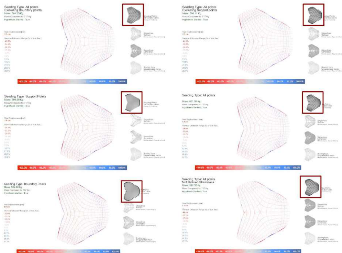
Figure 3: Structural Analysis of meshes with different seeding and refinement
