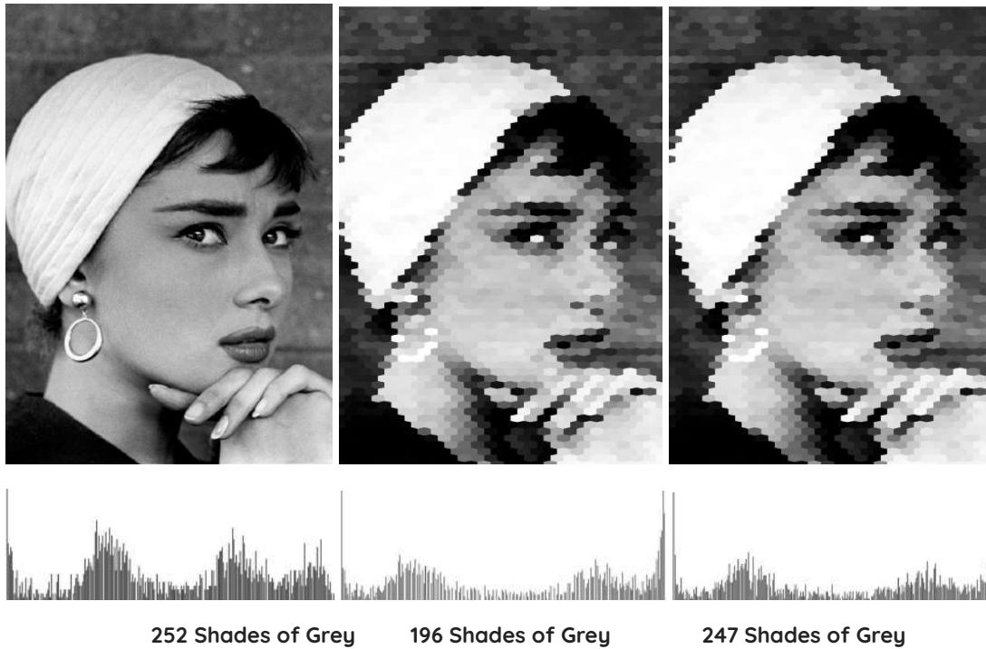
Fig1: Graphs showing the shades of grey that exist in each image respectively: Original image(a) the result from the image sampler(b) and the image sampled using the mean colors on each pixel(c)
