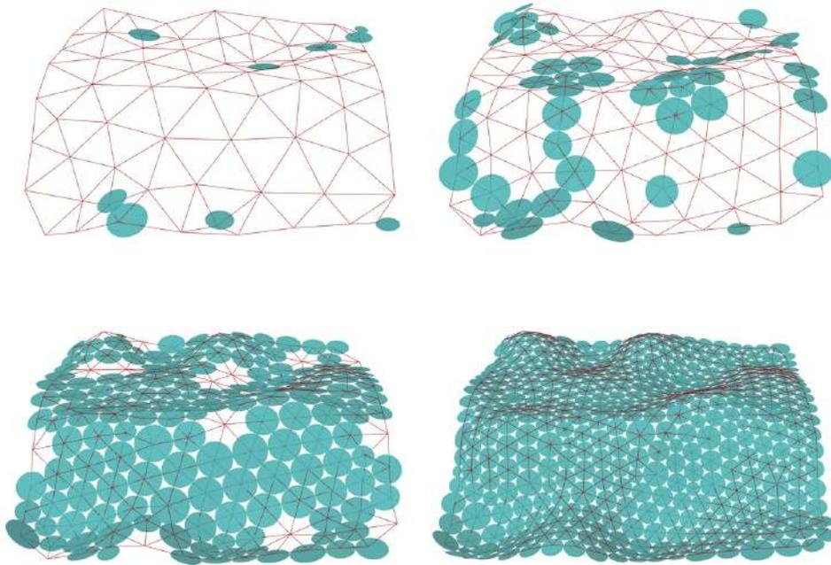
Figure 7: Adaption of a surface into a triangular mesh suitable for circle packing
