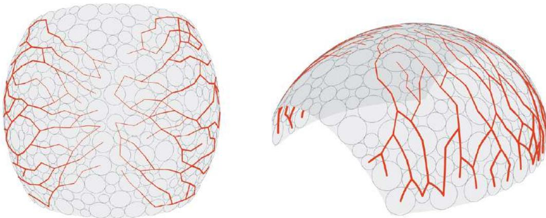
Figure 35: Visualization of load paths
