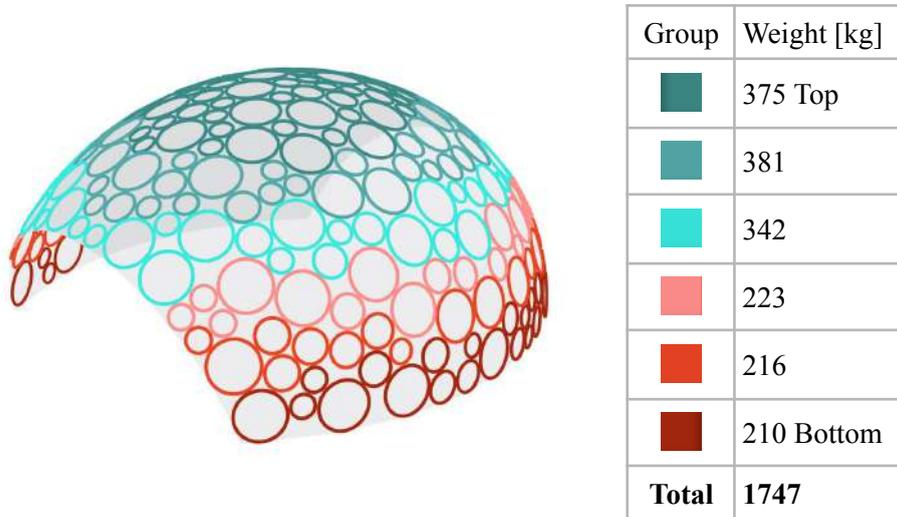
Figure 34: Order of assembly and weight estimates per section
