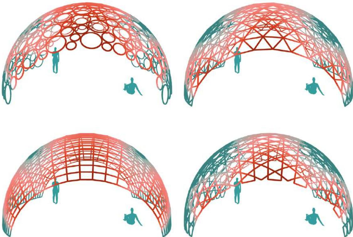
Figure 38: Left to right, top to bottom, Circle Packing, Tri Mesh, Quad Mesh, and Kagome
