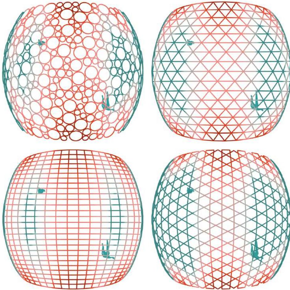
Figure 39: Left to right, top to bottom, Circle Packing, Tri Mesh, Quad Mesh, and Kagome
