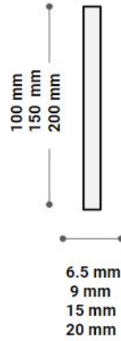
Figure 16: Planks sections chosen to test each gridshell.
