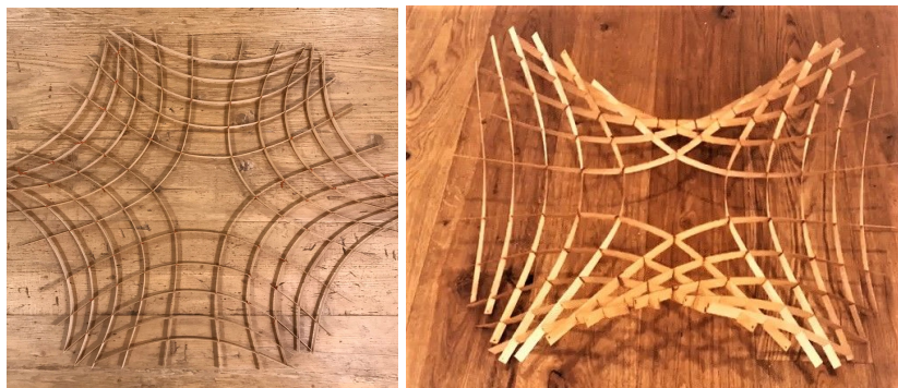
Figure 57: Enneper class 3 model fabrication after and before flattening
