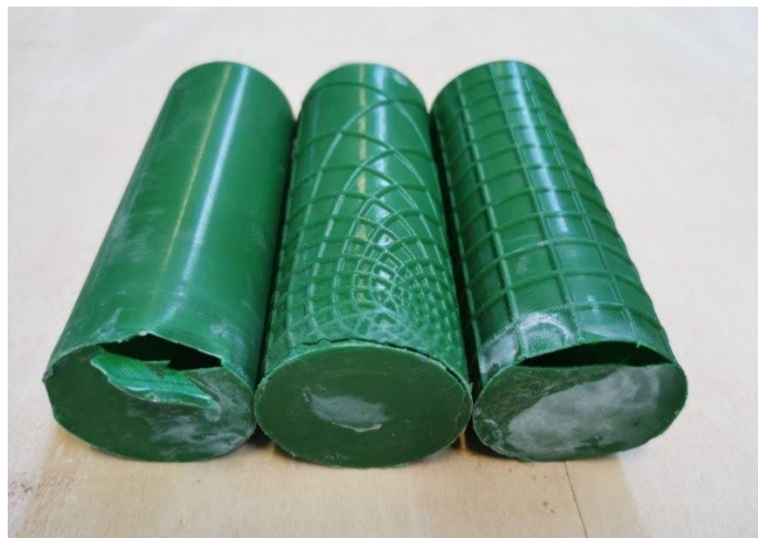
Figure 14: All the test objects failed from lower end bottom
