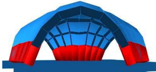
Figure 15: Panels in red on the boundary touch the ground just with one edge.
