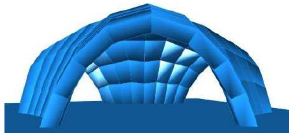
Figure 27: Three entries bottom panels completely touch the floor.
